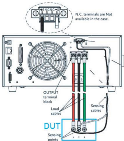
For high current output applications, the voltage drop caused by large current passing through the load cables will affect the measurement results. The ASR-2000 series provides the remote sense function that can sense the voltage drop of the DUT to the ASR-2000 series and the DUT will be compensated by the ASR-2000 series. The maximum voltage that the remote sense function can compensate is 5% of the output voltage.
