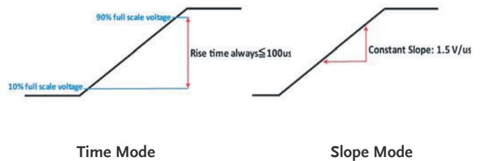
The ASR-2000 series can set the Slew Rate Mode to determine the rise time of the voltage according to the test requirements of the DUT. Slew Rate Mode provides "Time" and "Slope" modes. When setting "Time" mode, ASR-2000 can increase output to 10~90% of the set voltage within 100 $\mu$ s; and when selecting "Slope" mode, ASR-2000 increases output voltage by a fixed rising slope of 1.5V/ $\mu$ s until reaching the set voltage value.
